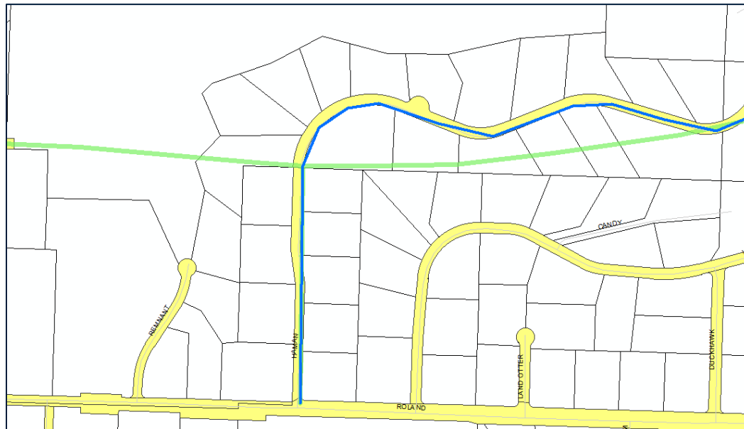
Figure 20: An example of the existing conditions analysis process. A planned corridor from the 1991 Road Plan (green) has a different built alignment (blue) and right-of-way (yellow) than proposed in the plan. This is due in part to on-the-ground topographical conditions and an alternative subdivision design accepted by the FNSB Platting Board that met the same requirements as the planned corridor. Source: PDC Engineers.
