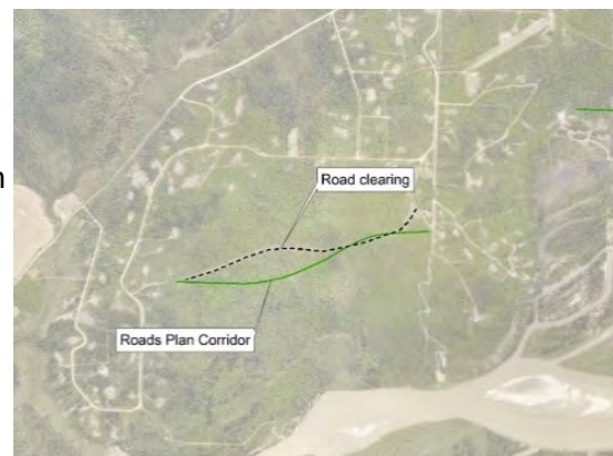
Figure 2: An example of a difference in the location of a planned road corridor in the 1991 Roads Plan versus the physically constructed road, likely due to topography. Source: PDC Engineers.
